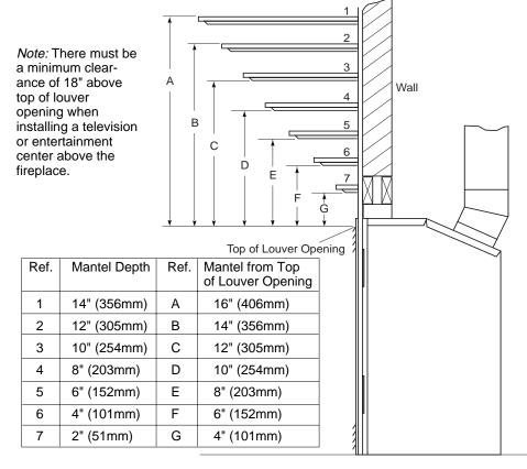
Figure 7 - Clearances for Combustible Mantels
